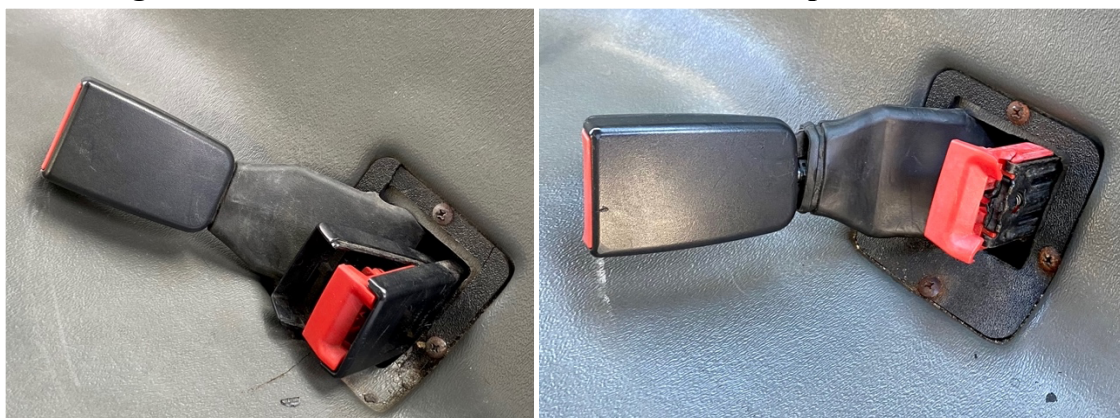
Figure 2: Images of Broken Seatbelt Mechanisms in Two Transport Vehicles
